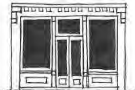
Mid to Late 1800's Boldly Decorated Cornice Cast Iron Columns Large Display Windows
